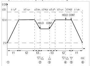
Ramp parameters: Output Quantity: U (range 0 ... 15 V), 5 $\pm$ Rrt = 2 V, Erd = 10 V,  $\pm$  I = 5 s,  $\pm$ Z = 8 s,  $\pm$ Z = 5 s, rEPERL for periodic ramps
