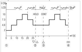
Interval parameters: Output Quantity: U (range  $0 \text{ V} \dots 15 \text{ V}$ ), SEArL = 2 V, End = 10 V, number of interval steps SEEPS = 3, E I = 5 s, PadE = Ruba
