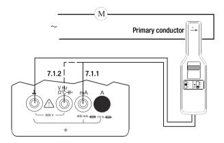
When reading the measured values in V, consider the transformation ratio of the transformer and the fact that the display shows current values as well as the additional display error.
