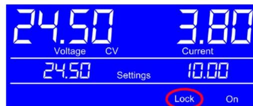
Lock condition remains until you deactivate it by pushing button **Lock** again, even if you would switch to remote control in-between and return from it, or switching the device off. The lock is not saved when switching the device off.
