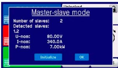
Tapping INITIALIZE will cause the master to search again for slaves and then to configure itself by setting all necessary parameters. If more than one correctly configured unit is found then this screen will show the number of slaves and the combined total current and total power.
