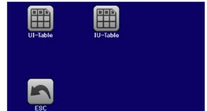
If the file naming, path and file content specifications are not met, the file is either not recognized at all or rejected. So it is, for example, impossible to load an UI table (file name starts with UI) for the IU function and vice versa. The USB drive may contain multiple files of which up to 10 are listed as a selection before loading.
