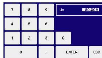
Decimal values are set by tapping the point key. For example, 54.3 V is set with **5** **4** **.** **3** and **ENTER**.
